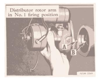
9. Position the ignition unit distributor arm and drive shaft lug (A) for firing number one cylinder. Install the ignition unit on the engine, meshing distributor lug (A) and governor drive slots (B).
