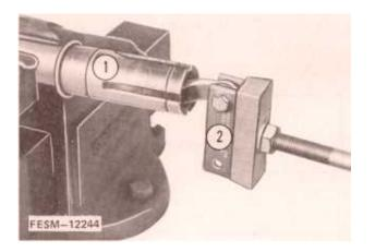
9. To remove the innermost bearing, use a slide hammer with only one appropriate length leg as shown.
