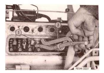
4. Compress the valve springs with a suitable tool and remove the valve spring seat keys (1). Be careful not to compress the springs more than necessary as they can be distorted.
