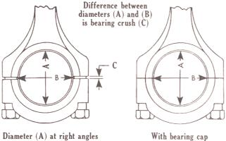
Diameter (A) at right angles to parting lines greater than diameter (B)
