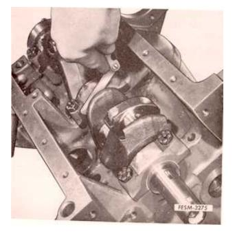
present between the bearing surface and the crankshaft journal. Measure the thickness with a micrometer or match the flattened Plastigage at several points (on either the bearing insert or the crankshaft), with the corresponding graduation on the Plastigage envelope, which indicates the clearance in thousandths of an inch. Running clearance must be .002 to .003 inch.
