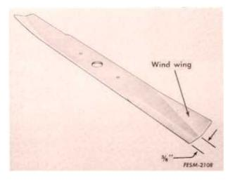
The cutting blade must be kept sharp at all times. The blade can be removed from the mower and sharpened on a grinding wheel.
