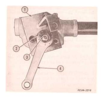
5. Install the lock nut (2) and tighten securely. Stake the nut into a housing slot (3).
