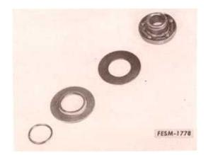
Observing the operation of the valves prior to tear-down of the engine is beneficial in preventing unnecessary checking of worn rotators. Mark the valves with a pencil as movement is relatively slight.
