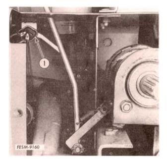
The PTO safety starting switch is spring loaded to complete the circuit as long as the PTO is disengaged.
