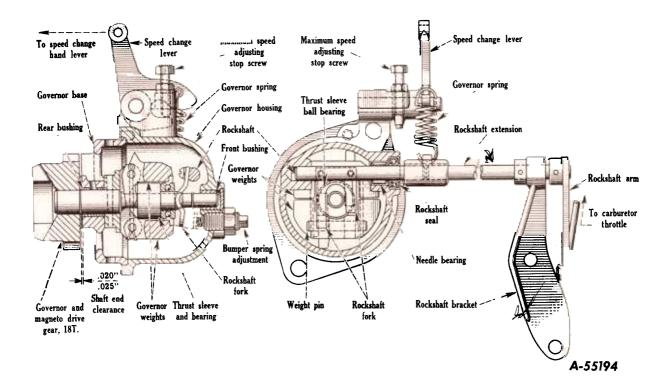
d. Advance operators speed change lever for a few seconds and again idle the engine, rechecking adjustments for specified low idle speed and smoothest operation.
