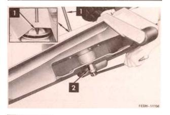
1. Pin-25.4 mm (1/2 inch) diameter 2. Removing blade nut
