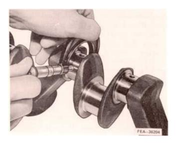
8. Remove the connecting rod bearing cap nuts and bolts and remove the caps. Push the piston and rod assemblies to the top of their travel.
