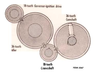
3. Install the key in the crankshaft if it was removed. Heat the crankshaft gear and install the gear, being sure the single timing mark of the camshaft gear and the single mark on the crankshaft gear are aligned.
