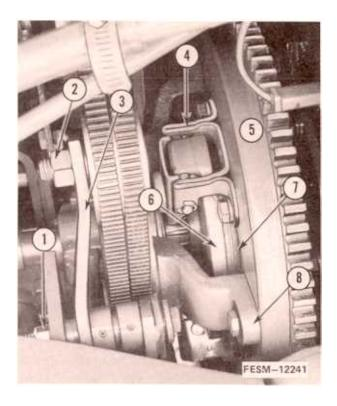
4. Relieve the clutch belt tension by pushing in on the idler tension arm nut with a 3/4 inch wrench and then slip the drive belts off the tension arm pulley.
