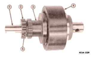
6. Install the low gear drive plate (3) and planet gears on the shaft (1) and in the main gear housing (4).
