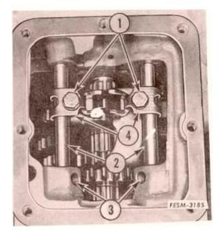
6. Shift the transmission into the neutral position and remove the shifter fork set screws (1).
