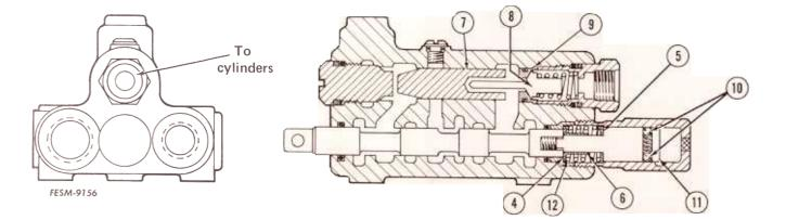
Hydraulic control valve cross section.
