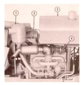
1. Remove the pipe plug in the water inlet elbow and drain the coolant.
