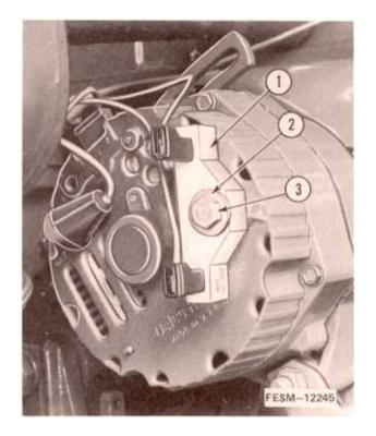
The resistor unit on the 184 tractor models, serial no. U046614 and above, requires a longer bolt and a plain washer instead of a lockwasher. The plain washer should be located between the bolt head and the resistor unit. Torque should not exceed 9-11 N·m (80-100 in. lbs.) to reduce the possibility of breakage of the ceramic resistor.
