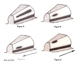
(d) Adjust the drive gear lateral position by removing shims from one side and installing the <u>shims</u> removed on the <u>opposite side</u>.
