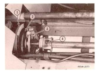
6. Install the pressure plate (3) and clutch disc assembly.
