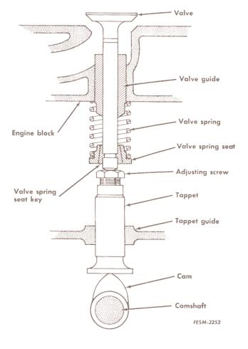
5. Remove the valves, valve spring seats and valve springs. Be sure to keep valves in order so they may be installed in the same port.
