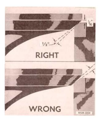
Grinding of valves to an interference angle provides line contact of the valve face to the seat for the first few hours of operation, allowing the valve and seat to 'wear in'' to a good tight contact. Interference angle has the effect of increasing the pressure per square inch on the seat, thus causing any deposits which cling to the face or seat to be squeezed out of the way and eventually blown out.
