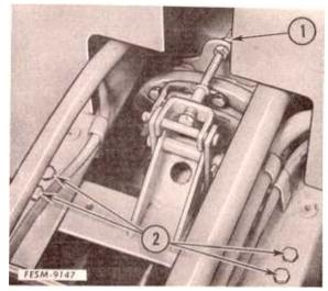
2. Remove the Allen head bolt from the clutch shaft coupling and slide the shaft ahead.
