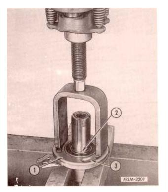
5. Compress the load spring and remove the snap ring retainer (2).
