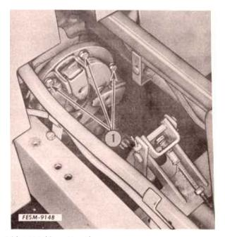
4. Remove the six bolts securing the pressure plate assembly to the input flywheel. Remove the pressure plate assembly and the clutch disc.
