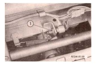
The safety starting circuit on early production tractors consisted of a main clutch safety starting switch. Later production tractors are equipped with safety starting switches on both the main clutch and the PTO.
