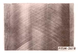
Use a good single point boring bar with a sharp tool and bore all cylinders the same size, to within .002 to .001 in. of the desired finished oversize to permit finishing honing operations.
