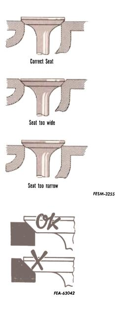
to clear away grinding dust. Grind the seat sufficiently to provide an even, smooth surface.
