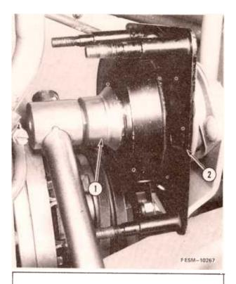
8. Install a breaker bar and 1-5/8 in. socket to the LH threaded field bearing nut and secure to the tractor frame with twine or wire.
