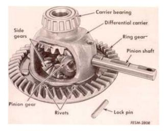
4. Assemble the side gears and the pinion gears in the differential case assembly.
