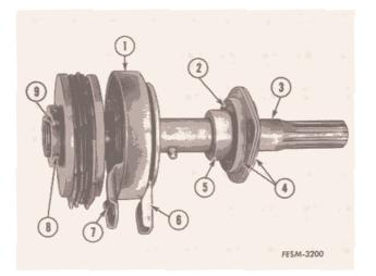
10. Install the bearing flanges (4),locking collar (5) and shaft ball bearing(2). Do not tighten the locking collar at this time.
