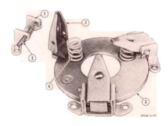
Check the bushing in the pressure plate for wear or damage. Replace if necessary.
